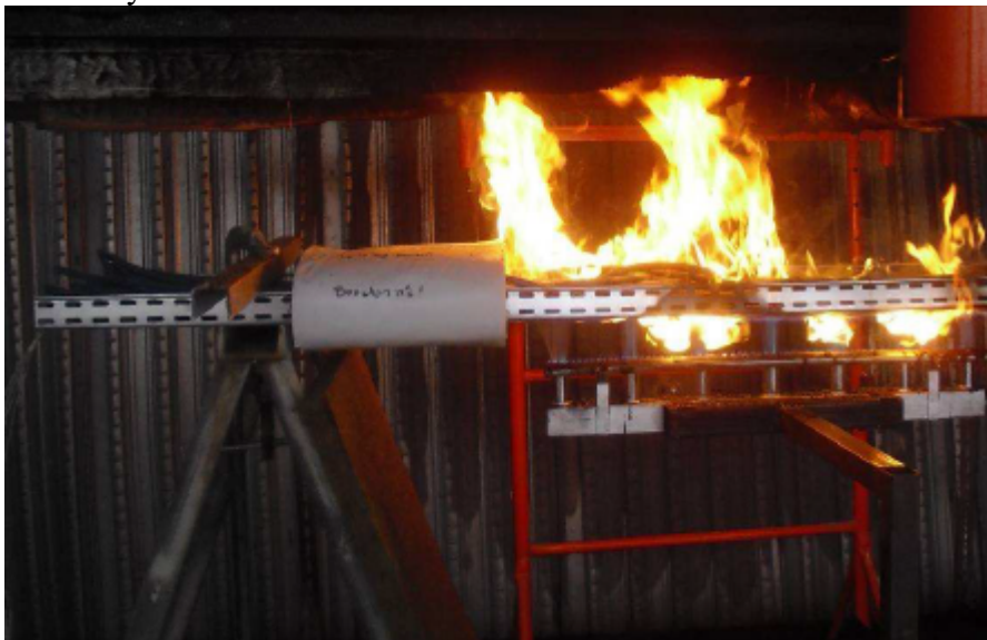
Figure 5.4.5.1 Configuration of cable trays with fire screen.
